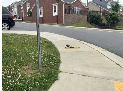
Figure 11 Measurement of Curb Ramp Slopes
