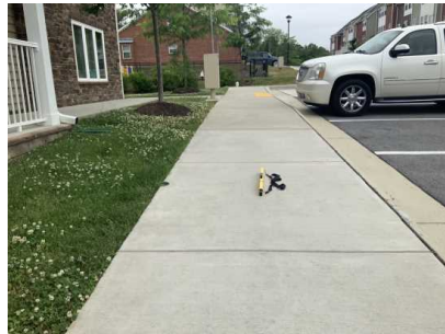
Figure 11 Measurement of Curb Ramp Slopes
